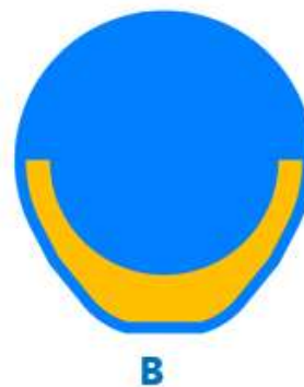
Contact shape Active area: 23µm diameter, ~425 µm 2
