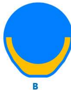
Contact shape Active area: 23 \mu\text{m} diameter, \sim 425 \mu\text{m}^2
